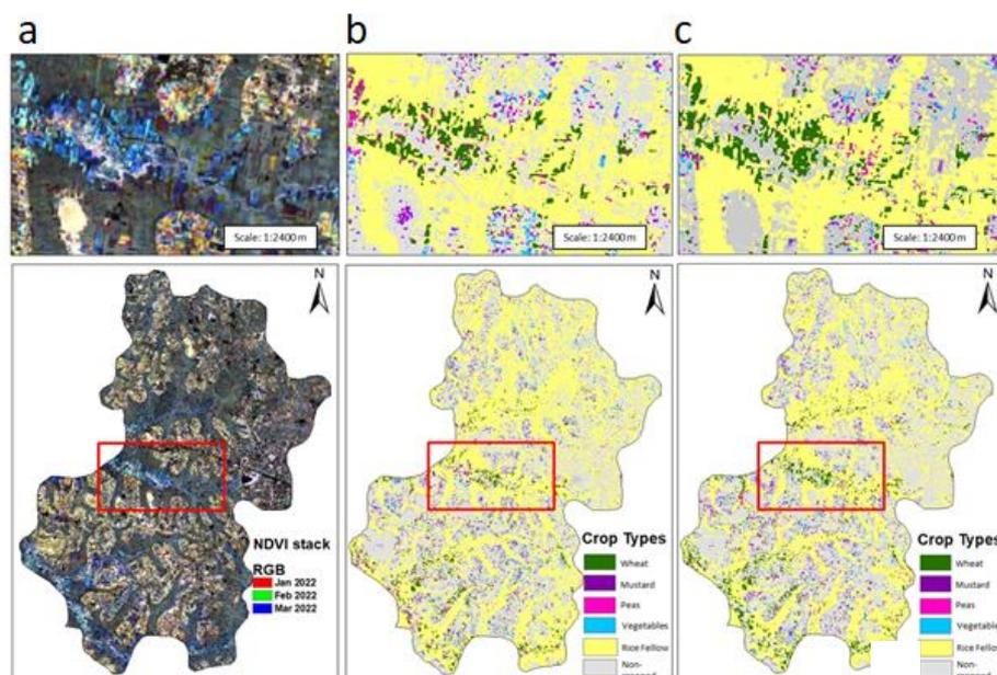
**Fig. 3** Rabi cropped type classification map: (a) NDVI composite: Red- January 20 2022; Green- February 2022; Blue- March 2022 (b) Classified using RF classifier. (c) Classified using 3D-CNN
